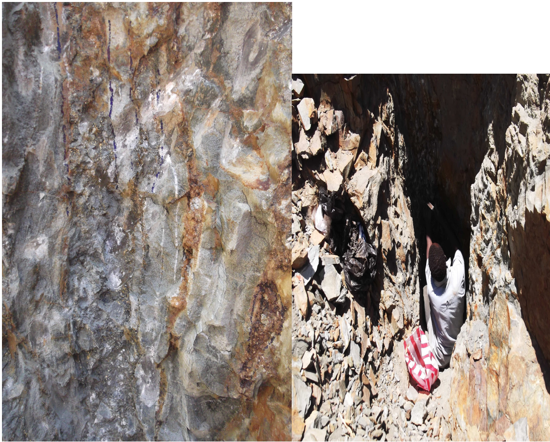
Fig10. Vertical multiple copper veins of varying width up to 50cm, right ; taking samples
