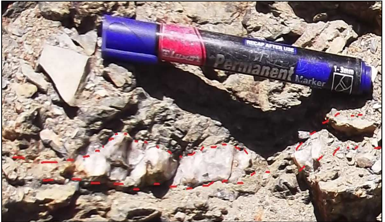
Fig12. Gold Mineralized quartz vein along strongly sheared metasediment revealed 0.3g/t
